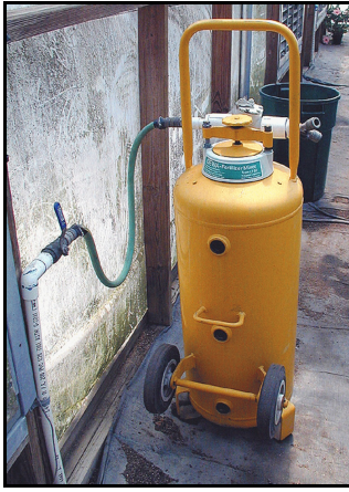
Figure 6. Gewa injectors are available in several sizes ranging from 4 gallons to 26 gallons. Depending on the model, they have proportioning ratios of 1:100 up to 1:300. The 15 different settings, 1:300 to 1:20 on the valve, are accurate to within 4 percent. A thick steel tank makes up the bulk of the Gewa. A system water flow of 1.6 gpm up to 88 gpm and system pressures up to 125 psi are required. The injectors are made with wheels and are easily movable.
