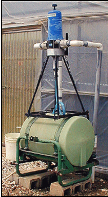
Figure 4. Maximum flow rates for DosMatic injectors range from less than 1 gpm to 100 gpm with ratios from 1:10 to 1:4000 on various models. The injection ratio can be adjusted while in use. A wide range of combinations of water flow and injection ratios can be accommodated, e.g., low flow and low injection, low flow and high injection to high flow and low injection, and high flow and high injection.
