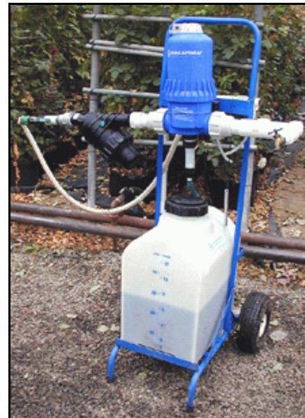
Figure 3. Maximum flow rates for Dosatron injectors range from 7 gpm to 264 gpm for various models, with ratios ranging from 1:50 to 1:500 for smaller flow rates, from 1:50 to 1:500 or 1:1000 for larger flow rates. The ratio can be easily adjusted on the outside of the injector. Dosatron injectors may be installed in a variety of system configurations in addition to being put directly in the water line. Special configurations allow flushing clean water (by-pass), injecting multiple solutions (series), and increasing water flow (parallel). Consult technical experts or check the Dosatron website (Table 4) for installation configurations.
